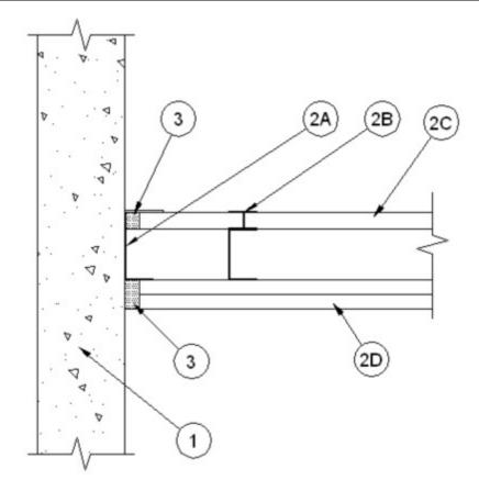
1. Concrete Wall Assembly — Min 4-1/2 in. (114 mm) thick reinforced lightweight or normal weight (100-150 pcf or 1600-2400 kg/m³) structural concrete. Wall may also be constructed of any UL Classified Concrete Blocks\*.
