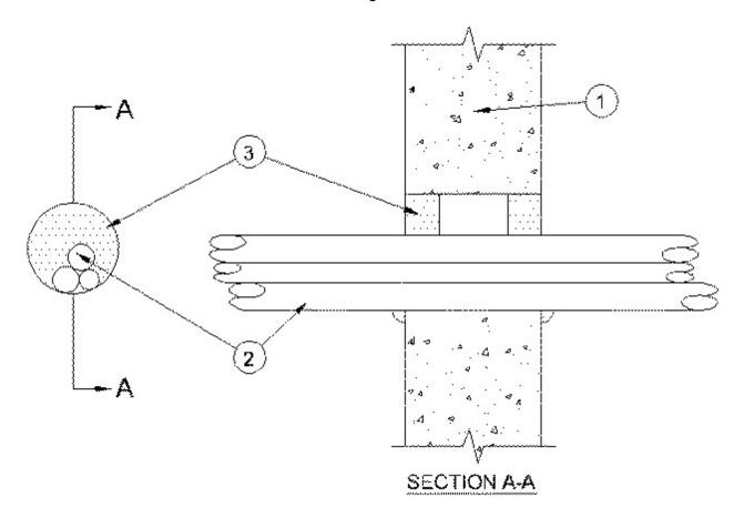
1. Wall Assembly — Min 6 in. thick reinforced lightweight or normal weight (100-150 pcf) concrete. Wall may also be constructed of any UL Classified Concrete Blocks\*. Max diam of opening is 4 in.
