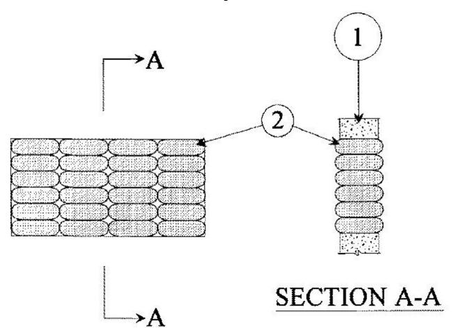
1. Wall Assembly — Min 5 in. thick reinforced lightweight or normal weight (100-150 pcf) concrete. Wall may also be constructed of any UL Classified Concrete Blocks\*. Max area of opening is 288 sq in. with max dimension of 24 in.
