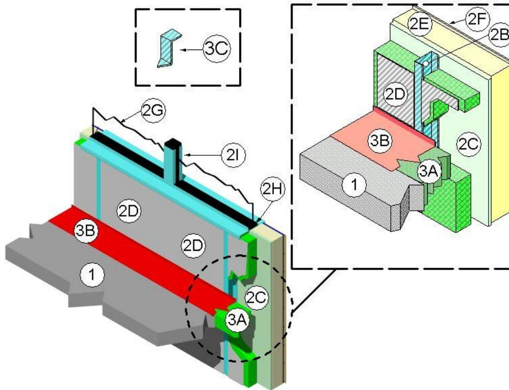
1. CONCRETE FLOOR ASSEMBLY: Two-hour rated concrete floor assembly made from either lightweight or normal weight concrete with a density of 100 to 150 pcf, having a min. thickness of 4-1/2 in. at the joint face. When a longitudinal recess (blockout) is required to contain an architectural joint system, increase concrete floor assembly thickness to
