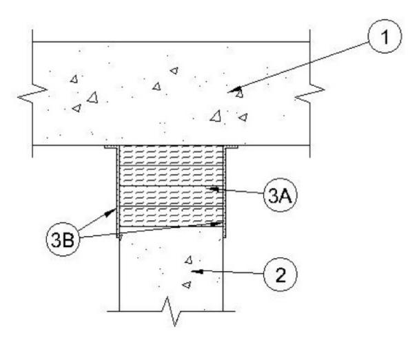
1. **Floor Assembly** — Min 4-1/2 in. (114 mm) thick reinforced lightweight or normal weight (100 - 150 pcf or 1600-2400 kg/m³) structural concrete. Floor may also be constructed of any min 6 in. thick UL Classified hollow-core **Precast Concrete Units\***.
