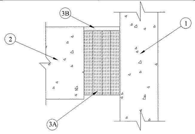
1. **Wall Assembly** — Min 6 in. thick reinforced lightweight or normal weight (100 - 150 pcf) structural concrete. Wall may also be constructed of any UL Classified **Concrete Blocks**\*.
