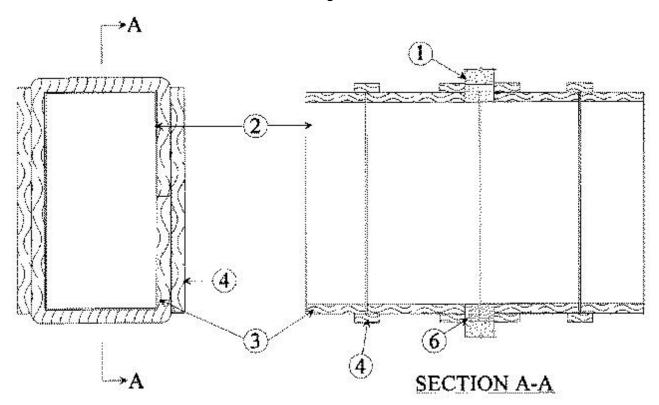
1. Floor or Wall Assembly — Min 4-1/2 in. (114 mm) thick reinforced lightweight or normal weight (100-150 pcf or 1600-2400 kg/m<sup>3</sup>) concrete. Wall may also be constructed of any UL Classified **Concrete Blocks**\*. For rectangular ducts, max area of opening shall be 1936 in<sup>2</sup>, with max dimension of 44 in. (1118 mm), For round ducts, max diam of opening shall be 44 in. (1118 mm). For oval shaped ducts, max dimension of opening shall be 44 in. (1118 mm) by 14 in. (356 mm).
