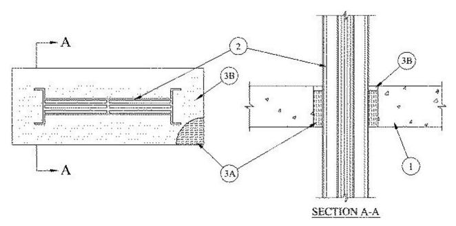
1. **Floor or Wall Assembly** — Min 4-1/2 in. thick reinforced lightweight or normal weight (100-150 pcf) concrete floor or min 5 in. thick reinforced lightweight or normal concrete wall. Wall may also be constructed of any UL Classified **Concrete Blocks**\*. Max area of opening is 360 sq. in. with max dimension of 30 in.
