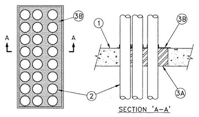
1. **Floor or Wall Assembly** — Min 4-1/2 in. (114 mm) thick reinforced light weight or normal weight (100-150 pcf or 1600-2400 kg/m³) concrete. Wall may also be constructed of any UL Classified **Concrete Blocks**\*. Max area of opening is 864 sq. in. (0.56 m²) with max dimension of 48 in. (1.22 m).
