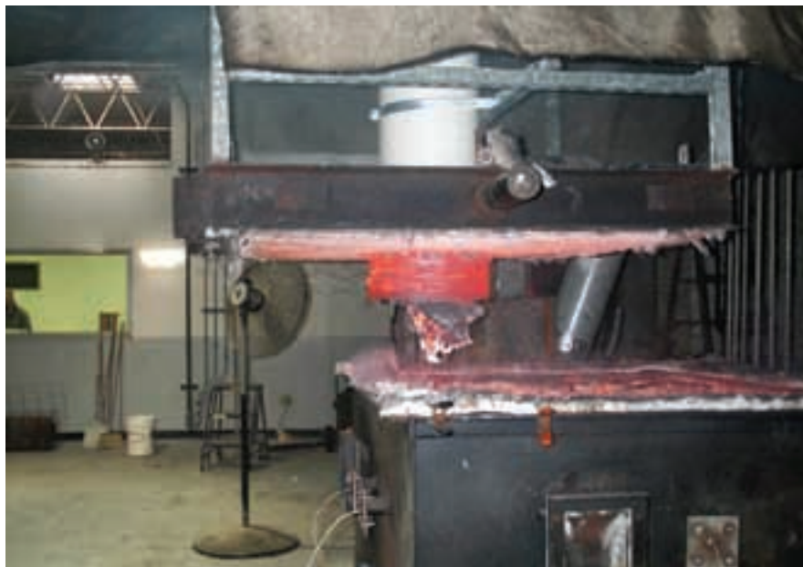
A fire test is conducted on 12-inch PVC DWV pipe. Product testing is the responsibility of the firestop manufacturer. (Photo courtesy of Randy Clark)
